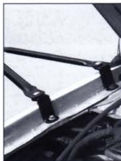
Fender-mounted "Z" brackets.
