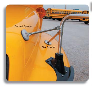
Includes two 74-3300-H Curved Surface Mount Assemblies and two 74-300-F Flat Surface Mount Assemblies. The Mirror Lite Solar Eclipse<sup>™</sup> meets FMVSS 111 as certified on IC buses and is an acceptable upgrade cross-view mirror system.
