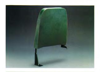
C.E. White barriers are designed with a deep recess in the knee impact area. This feature provides for additional seat installation without sacrificing passenger comfort and safety.
