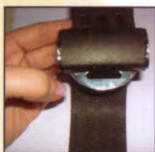
lift up on tilt-lock to adjust tether
