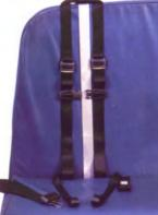
The KidCam<sup>™</sup> Harness secures around a bus seat equipped with standard lap-belts.
